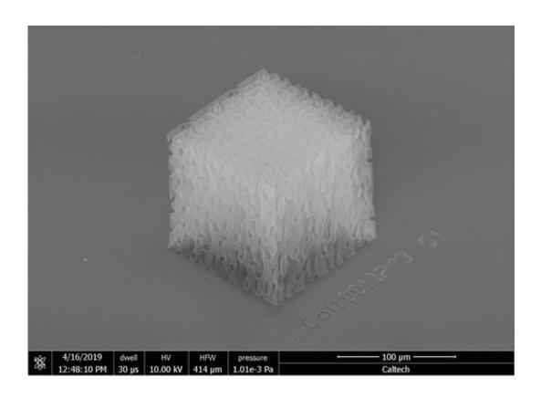
Engineers grew cubes of nanoarchitected material to test its strength and resilience. Credit: Greer Lab/Caltech
