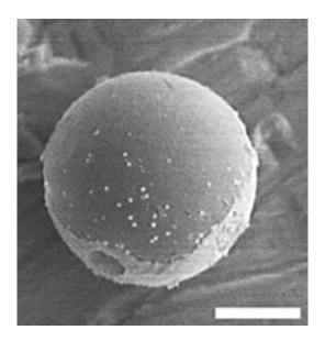
For the first time, a micromotor (shown above) was powered by "engines" that respond to three different stimuli: catalytic (bubbles), light and magnetic. Scale bar, 10 µm. Credit: Adapted from *Chemistry of Materials* 2020, DOI: 10.1021/acs.chemmater.9b04873
