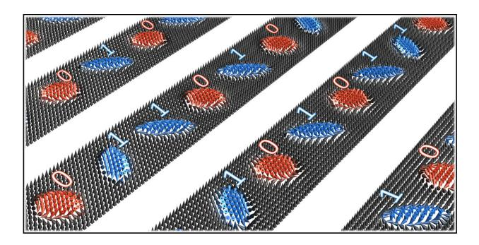
Schematic representation of the magnetization in an advanced racetrack memory data storage. Skyrmions (blue) and antiskyrmions (red) constitute the '1' and '0' bits, respectively. Credit: Dr. Börge Göbel/MLU
