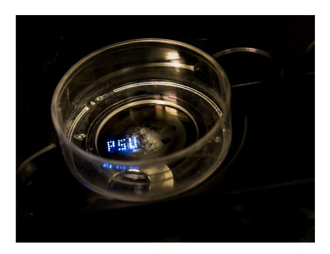
PSU aspiration bioprinted on the bottom of a glass Petri dish. The spheroids of tissue can be seen. Credit: Ozbolat's Lab/Penn State
