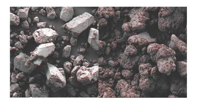
Examples of two different TATB crystal structures synthesized under different conditions, shown at identical magnifications. Credit: Lawrence Livermore National Laboratory
