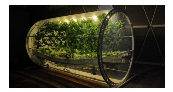
The 18-foot long, 7-foot diameter lunar greenhouse chamber is equipped as a prototype bioregenerative life support system. Credit: Gene Giacomelli/Department of Biosystems Engineering
