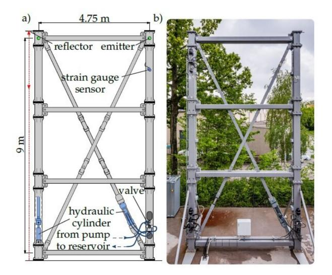
The researchers applied their new camera-based method for measuring building deformations to monitor very small movements of an adaptive building
