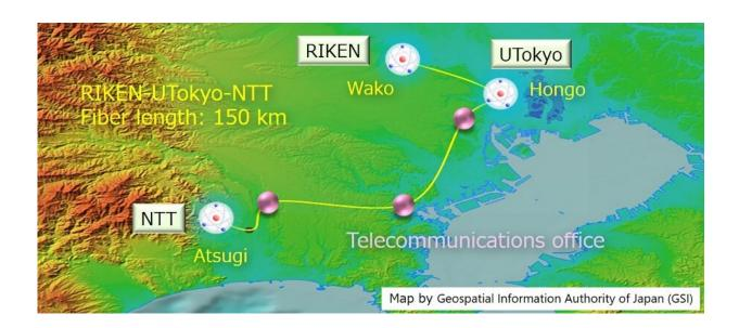
Researchers connected three laboratories in a 100-kilometer region with an optical telecommunications fiber network stable enough to connect optical atomic clocks. Credit: Tomoya Akatsuka, Nippon Telegraph and Telephone Corporation
