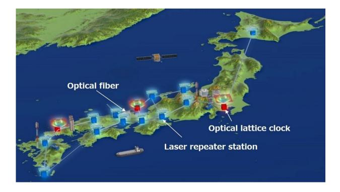
The new low-noise network could be expanded to create an optical lattice clock network in Japan (concept pictured). Credit: Tomoya Akatsuka, Nippon Telegraph and Telephone Corporation
