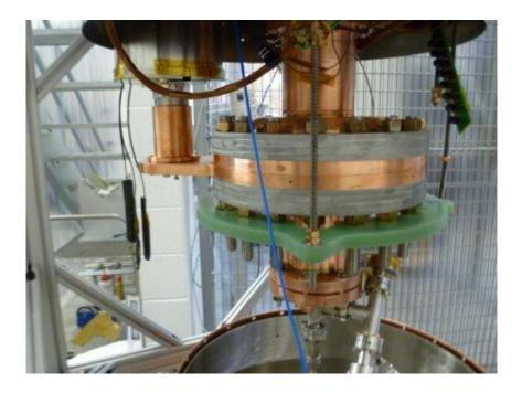
Copper/Niobium/NiobiumTin cavity connected to the cryocooler. Credit: US Department of Energy
