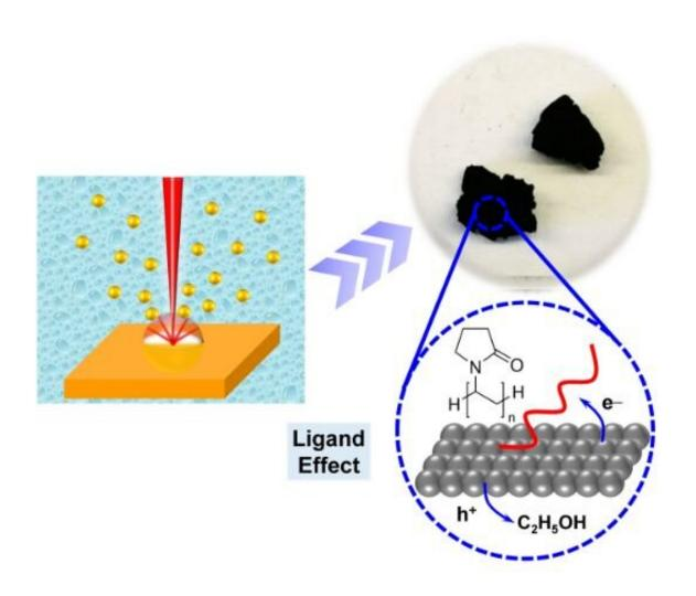
In light of cleanliness of laser-produced metal nanoparticle precursors, surfaceclean noble metal aerogels are created. The intrinsic electrocatalytic properties
