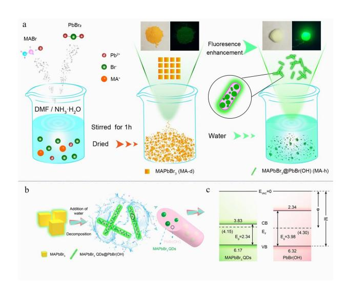
a) Schematic diagram of the synthesis process for MAPbBr3@PbBr(OH). b) Schematic illustration of the morphology evolution of the as-prepared MAPbBr3 perovskite. c) Energy level diagram of PbBr(OH) and inner QDs. Credit: by Kai-Kai Liu, Qian Liu, Dong-Wen Yang, Ya-Chuan Liang, Lai-Zhi Sui, Jian-Yong
