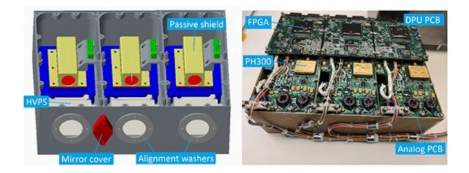
The HaloSat science payload is completely contained in a single aluminum subassembly. This subassembly is mounted inside the payload enclosure of the spacecraft bus. Credit: University of Iowa
