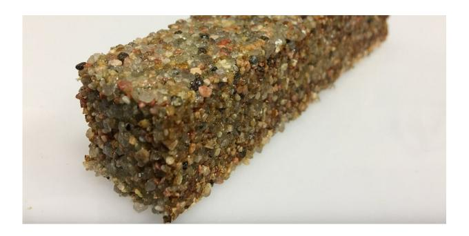
A block of sand particles held together by living cells. Credit: The University of Colorado Boulder College of Engineering and Applied Science, <u>CC BY-ND</u>
