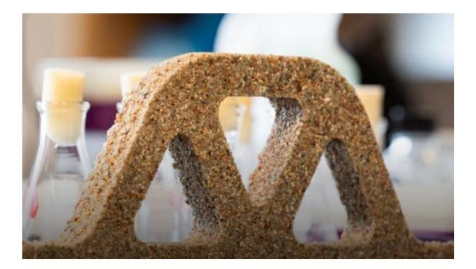
Living building materials can be formed into many shapes, like this truss. Credit: The University of Colorado Boulder College of Engineering and Applied Science, <u>CC BY-ND</u>
