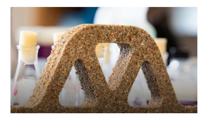
Living building materials can be formed into many shapes, like this truss. Credit: The University of Colorado Boulder College of Engineering and Applied Science, CC BY-ND
