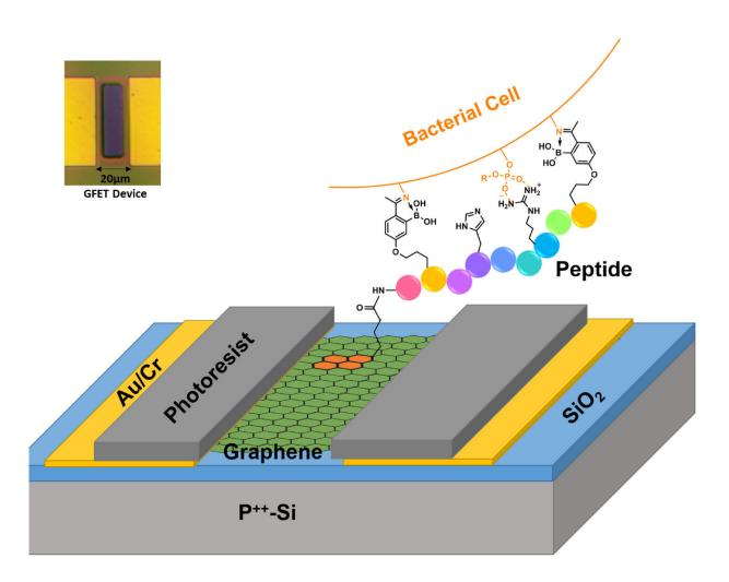
The difficulty and expense of determining the precise pathogen causing an infection is a key part of the complexity of antibiotic treatments. A team led by Boston College researchers has developed a prototype sensor that uses an atomdeep sheet of graphene and peptides to rapidly reveal which bacterial species is in a sample and whether it is antibiotic resistant. The graphene field effect
