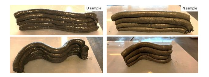
Tests to see the ability to form layers of a mixture of material with 3% urea (sample U) and another with 3% naphthalene, a common plasticizer (sample N) Credit: Shima Pilehvar et al. / *Journal of Cleaner Production*
