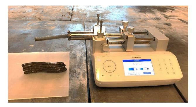
Device for printing 3D samples Credit: Shima Pilehvar et al./ Journal of Cleaner Production
