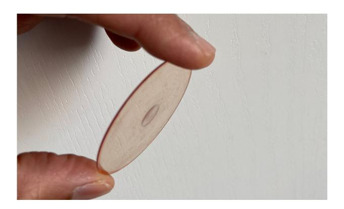
Using a single lens that is about one-thousandth of an inch thick, researchers have created a camera that does not require focusing. The new lens could drastically reduce the weight, complexity and cost of cameras and other imaging systems, while increasing their functionality. Credit: Rajesh Menon, University of Utah
