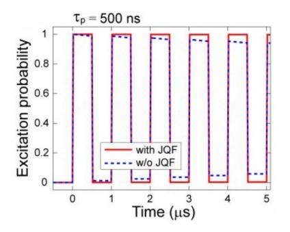
Time evolution of the excitation probabilities of the data qubit under successive application of pi-pulses. The red solid (blue dotted) line shows the results with (without) the JQF. Credit: Tokyo Medical and Dental University
