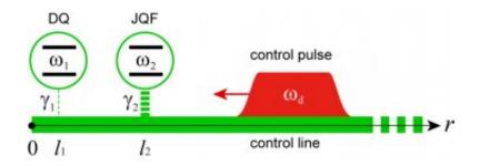
Schematic of a Josephson quantum filter (JQF). The data qubit (DQ) to be protected and the JQF are directly coupled to a semi-infinite waveguide, through which control pulses for the DQ are applied. Credit: Tokyo Medical and Dental University
