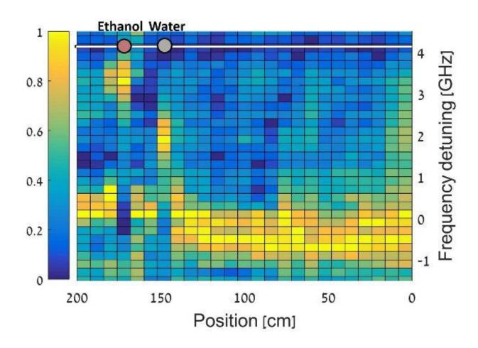
Researchers at Bar-Ilan University in Israel have demonstrated a new concept of optical fiber sensors that addresses a decades-long challenge: the distributed mapping of refractive index outside the cladding of standard fiber, where light does not reach. The sensor can be used for leak detection in critical
