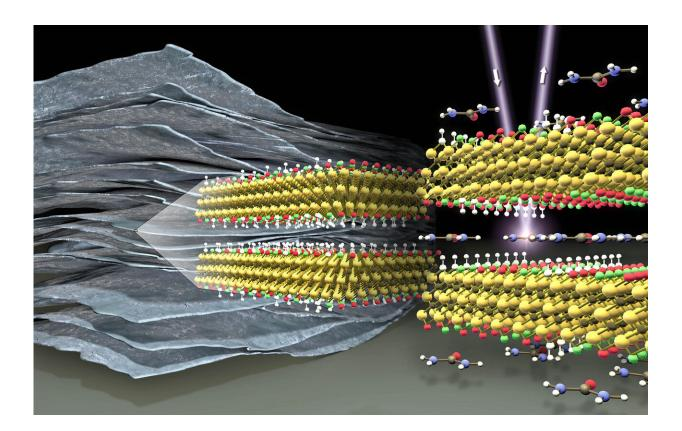
MXenes are 2D materials forming multi-layered particles (left) from which pseudocapacitors are made. Shining X-ray light on MXenes revealed changes of their chemical structure upon intercalation of urea molecules (right) compared to pristine MXenes (center). Credit: HZB/Martin Künsting
