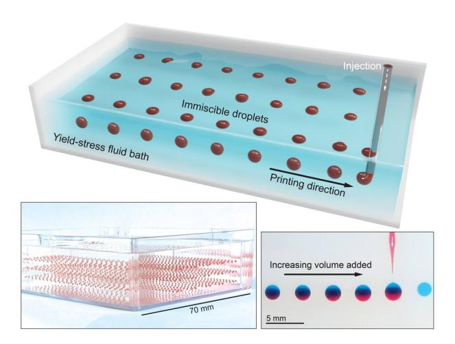
The new embedded droplet printing method suspends 3-D arrays of droplets in a uniquely isolated state that allows for precise processing and experimentation Credit: Singapore-MIT Alliance for Research and Technology (SMART)
