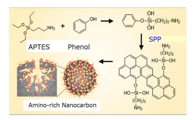
Synthesis process of nanocarbon adsorbent. Credit: Nagahiro Saito
