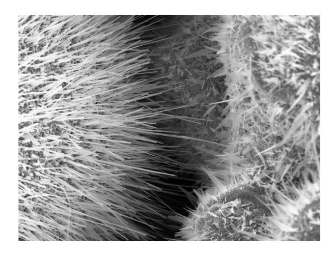
The sensor surface under the microscope: the research team grows tiny wires and spikes from metallic microparticles that are particularly good at trapping gas molecules. Credit: Working Group Functional Nanomaterials
