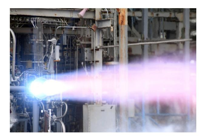
The 3D-printed thrust chamber assembly of the methane-fuelled M10 rocket engine passed its first series of hot firing tests at the NASA Marshall Space Flight Center in the USA during February 2020. The M10 engine will power the upper stage of future Vega evolutions from 2025. Credit: ESA/NASA
