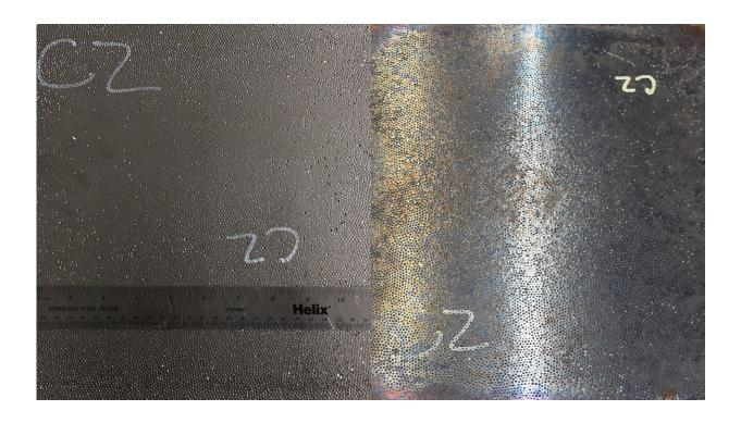
Steel-steel composite metal foam samples before testing (right) and after 100 minutes exposure to 825C (left). Credit: Afsaneh Rabiei, NC State University
