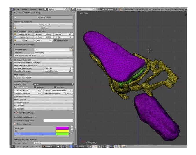
Figure 2Screenshot of the BlendGAMer tool shelf menu in 3D modeling software Blender. The user can call GAMer mesh conditioning, analysis, boundary marking, and tetrahedralization functions by clicking buttons and adjusting settings in the tool shelf. Shown on the right is a conditioned surface mesh of the CRU model. Credit: GAMer 2
