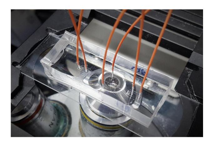
The chip device, called a spiral hydroporator, contains tiny fluid-filled channels. A fluid suspension of cells and target nanomaterials is delivered and removed via the orange tubes. Credit: Korea University
