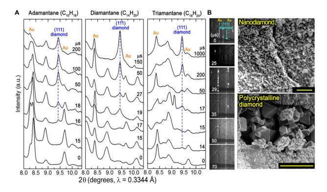
Onset timing of diamond formation from lower diamondoids. (A) In situ XRD patterns of three diamondoids as a function of increasing laser-heating duration. Nonlabeled peaks belong to the sample. (B) Cake integration of two-dimensional diffraction images highlighting the texture of diamond growth as a function of increasing laser-heating time. Representative SEM images of nanodiamond and polycrystalline diamond. Scale bars, 2 µm. Credit: *Science Advances*, doi: 10.1126/sciadv.aay9405
