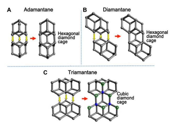
Mechanisms of diamond formation from lower diamondoids. (A) Two unpassivated adamantane molecules can only fuse to form a hexagonal diamond cage. (B) Two unpassivated diamantane molecules can only fuse to form a hexagonal diamond cage. (C) Two unpassivated triamantane molecules fuse to form a cubic diamond cage enabled by the quaternary carbon atoms (blue spheres) and surrounding tertiary carbon atoms (circled in green). Credit: Science Advances, doi: 10.1126/sciadv.aay9405
