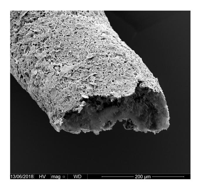
Close-up of a tubular structure made by simultaneous printing and self-
