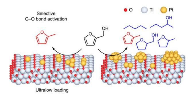
Scientists loaded single atoms of platinum (yellow) on top of titania, a compound containing titanium (grey) and oxygen (red). This catalyst selectively breaks a bond between a carbon and oxygen in furfuryl alcohol, a five-member ring-shaped molecule with an attached side group (structure in black). Credit: Brookhaven National Laboratory
