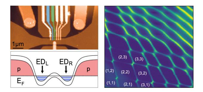
Atomic force microscope image, showing the gate layout of the device. The source (S) and drain (D) contacts are connected to the BLG through etched vias in the hBN. The gate stack contains split gates (SG) with a separation of 50 nm and on top, separated by Al2O3, six parallel finger gates with a gate separation of 50 nm and a width of 100 nm. The gates GL and GR (color coded) are used to control the QDs discussed in this work. Credit: Nano Letters
