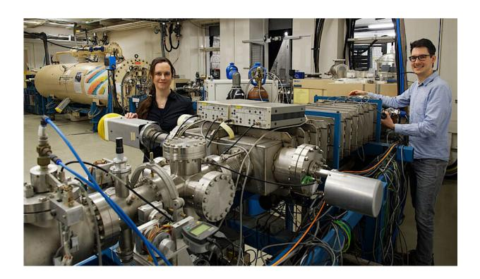
The Vienna Environmental Research Accelerator (VERA) was used to detect the ultra-trace concentrations of 233U and 236U (in the picture K. Hain with Master student M. Kern). Credit: M. Martschini, University of Vienna
