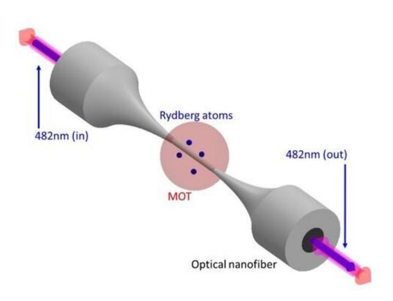
The scientists used a device called a magneto-optical trap (MOT) to capture and cool Rubidium atoms, which were then excited to a Rydberg state. Credit: Okinawa Institute of Science and Technology
