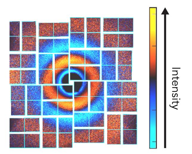
A diffraction pattern made by X-rays scattering off an iodine molecule into an detector at SLAC National Accelerator Laboratory. Hundreds of these patterns from the lab's X-ray free-electron laser were strung together to create a
