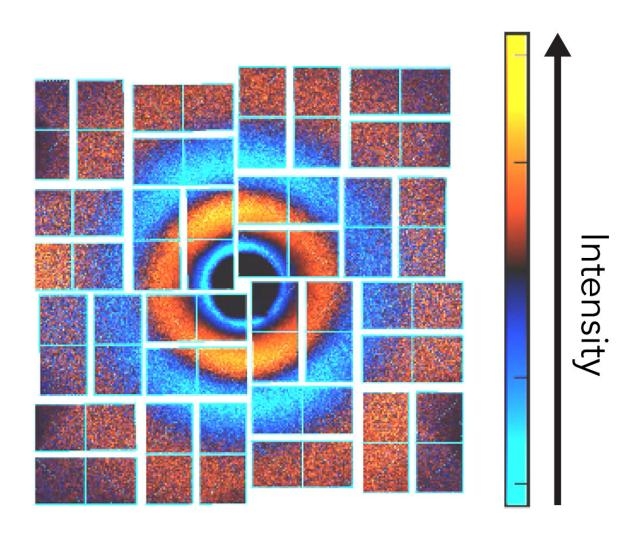
A diffraction pattern made by X-rays scattering off an iodine molecule into an detector at SLAC National Accelerator Laboratory. Hundreds of these patterns from the lab's X-ray free-electron laser were strung together to create a
