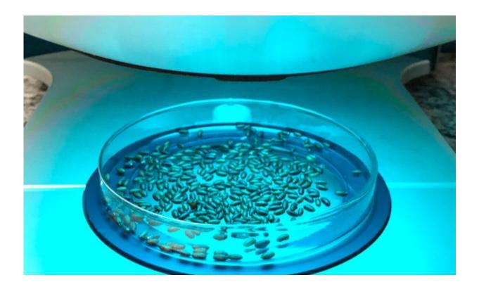
Picture of VideometerLab equipment performing reflectance imaging analysis on pupae of Anastrepha fraterculus. Credit: LRA /CENA-USP
