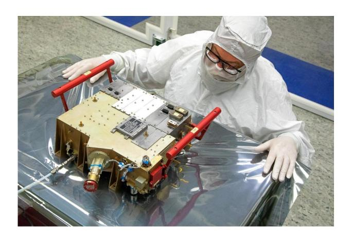
Southwest Research Institute packages its Ultraviolet Spectrograph (UVS) for delivery and integration onto the European Space Agency's JUICE spacecraft. As part of a 10-instrument payload to study Jupiter and its large moons, UVS will be used to study the composition and structure of the atmospheres of these bodies and how they interact with Jupiter's massive magnetosphere. Credit: Southwest Research Institute
