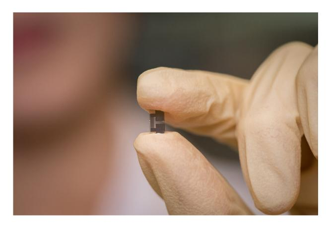
The device that the researchers developed is an integral part of the battery and works by emitting ultrasound waves to create a circulating current in the electrolyte liquid found between the anode and cathode. This prevents the formation of lithium metal growths, called dendrites, during charging that lead to decreased performance and short circuits in LMBs. Credit: David Baillot/University of California San Diego
