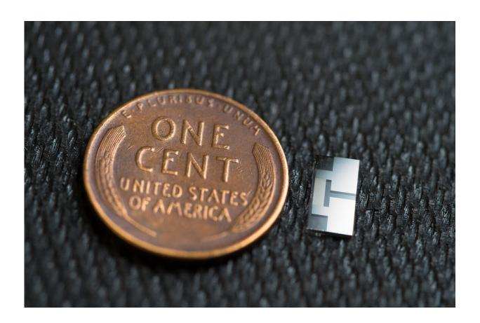
The device is made from off-the-shelf smartphone components, which generate sound waves at extremely high frequencies--ranging from 100 million to 10 billion hertz. In phones, these devices are used mainly to filter the wireless cellular signal and identify and filter voice calls and data. Researchers used them instead to generate a flow within the battery's electrolyte. Credit: David Baillot/University of California San Diego
