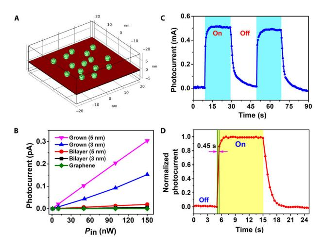
COMSOL simulation and transient photoresponse. (A) Schematic of COMSOL simulation of PQDs of size 3 nm grown on a graphene film. (B) Simulated photocurrent versus input power. (C) Transient photoresponse under light illumination on and off conditions. (D) Normalized photocurrent response to on and off illumination. Credit: Science Advances, doi: 10.1126/sciadv.aay5225
