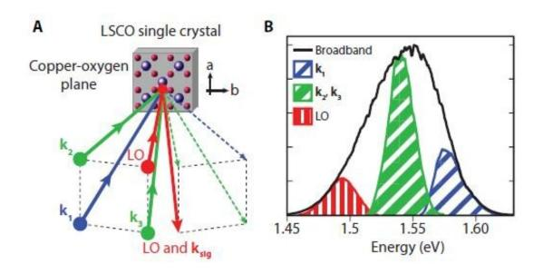
Three excitation pulses with wave vectors k1, k2, and k3 form three corners of a box with 4th pulse (local oscillation; LO) on the fourth corner. Credit: FLEET
