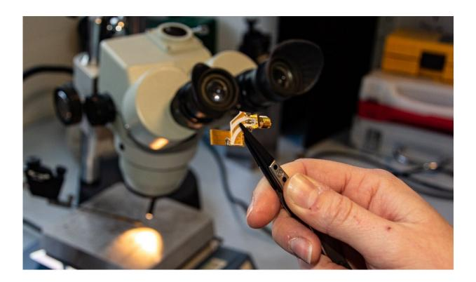
The terahertz quantum cascade laser on its mounting. A pair of tweezers shows how small the device is. Credit: University of Leeds
