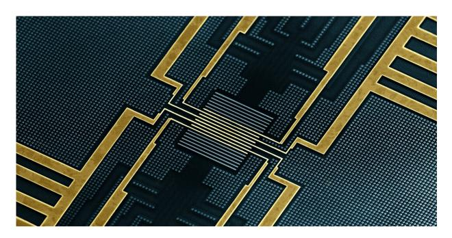
The chip produced by IMEC for the experiments at ETH. The tunnel junctions used to measure the timing of the magnetisation reversal are located at the centre (Image courtesy of IMEC). Credit: IMEC
