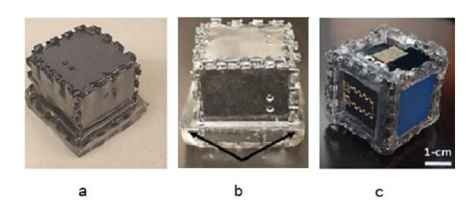
Steps to create a floating multidimensional integrated circuit: a) the MD-IC is encapsulated with a bio-safe polymer, b) with an asymmetric base to enable it to float but stay right-way up and c) with a solar cell on top and water sensors on the bottom. Credit: KAUST
