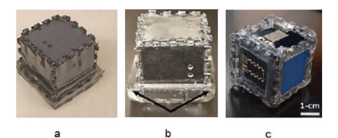
Steps to create a floating multidimensional integrated circuit: a) the MD-IC is encapsulated with a bio-safe polymer, b) with an asymmetric base to enable it to float but stay right-way up and c) with a solar cell on top and water sensors on the bottom. Credit: KAUST
