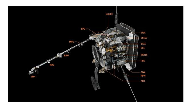
Labelled diagram showing a cutaway of Solar Orbiter's suite of ten science instruments that will study the sun. There are two types: in situ and remote sensing. The in situ instruments measure the conditions around the spacecraft itself. The remote-sensing instruments measure what is happening at large distances away. Together, both sets of data can be used to piece together a more complete picture of what is happening in the sun's corona and the solar wind. Credit: ESA/ATG media lab
