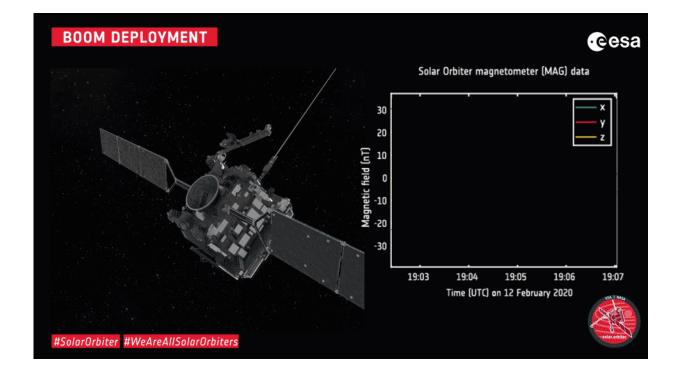
Data collected with the Magnetometer (MAG) instrument during the deployment of the instrument boom of ESA's Solar Orbiter spacecraft show how the magnetic field decreases from the vicinity of the spacecraft to where the instruments are actually deployed. Solar Orbiter was launched on 10 February 2020 from NASA's Kennedy Space Center in Cape Canaveral, Florida. The magnetometer's two sensors were switched off about 21 hours after liftoff, and
