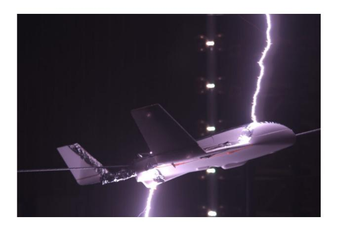
Side view of the 1-meter wingspan model plane used in the experiments with both positive and negative lightning. Credit: Carmen Guerra-Garcia
