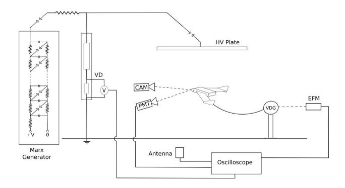
A schematic of the apparatus used to test aircraft charging and lightning strikes. Note the Van de Graaf (VDG) generator used to charge the model plane. Credit: Pavan, et al., 2020, JGR Atmospheres
