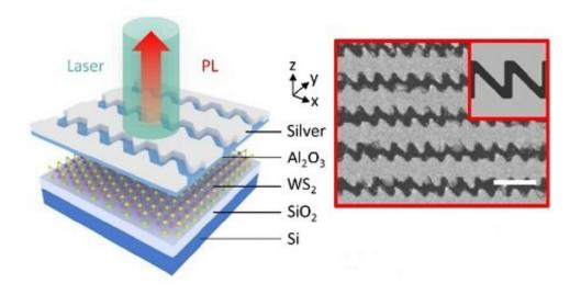
After excitation of the device with green laser light (green), coherent fluorescence occurs (red) thanks to the silver saw tooth (right panel). The scale bar is 500 nm. Credit: Illustration--Han and Ye, University of Groningen.
