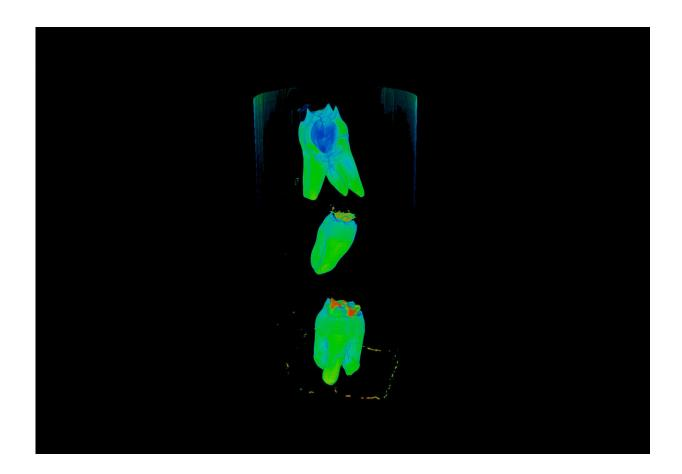
Neutron scattering at ORNL's High Flux Isotope Reactor was used to study the effectiveness of dental implants. Neutron imaging radiographs illustrate restorative materials bound to the tooth structure via Esteban Florez's experimental adhesive resins, which contain differing concentrations of metal oxide nanoparticles. Credit: ORNL/Hassina Bilheux
