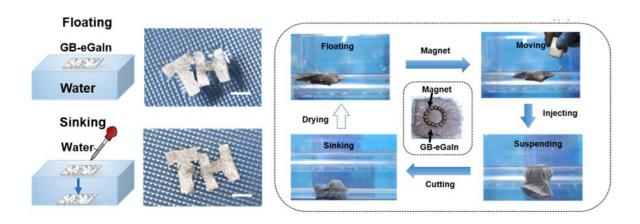
Figure 3. Floating behavior of GB-eGaIn in planar and 3-D structure. Credit: LIU Jing
