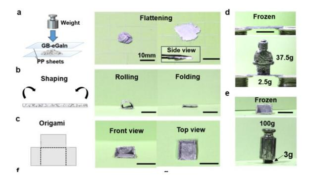
Figure 2. Planar Structure of GB-eGaI. Credit: LIU Jing
