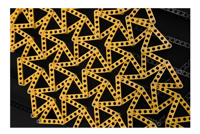
Scientists used a LEGO array to demonstrate how sound waves can propagate identically in different structures. Credit: V. Vitelli and M. Fruchart, University of Chicago
