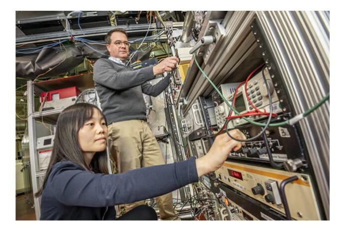
Meirong Zeng (left) and Kevin Wilson at Beamline 9.0.2 of the Advanced Light adjusting the Aerosol Mass Spectrometer to measure the degradation kinetics of lipids. Credit: Marilyn Sargent/Berkeley Lab
