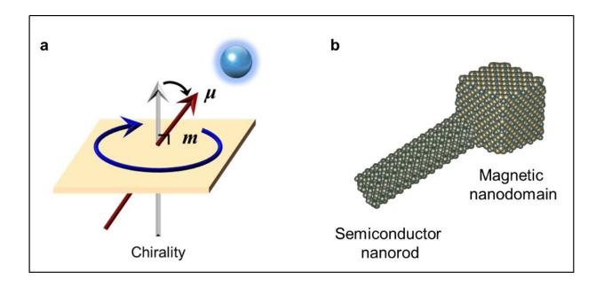
a, Schematic illustration of magnetically induced chiroptical activity. b, Model of materialized magnetite nanodomain at one apex of ZnxCd1-xS semiconductor nanorod. Credit: ZHUANG et al.
