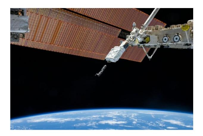
First of many CubeSats deployed from the International Space Station by the NanoRacks company in February 2014. The Nanoracks deployment system containing one or more CubeSats inside it is placed through JAXA's Kibo module's airlock. From here the module's robotic arm – the Japanese Experimental Module Remote Manipulator System – positions the deployer for safe orientation away from the station for deployment. Credit: Nanoracks
